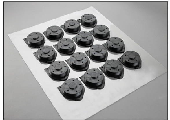
A platform of black > ABS parts that were built in .010" layers for a low volume production application.
