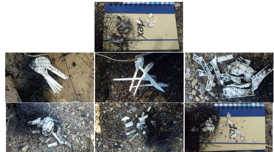
Figure 3: Disintegration of crystallized PLA HH cutlery as tested at Specialized Environmental Technologies Inc. Composting facility, MN from Day 1 through Day 18
