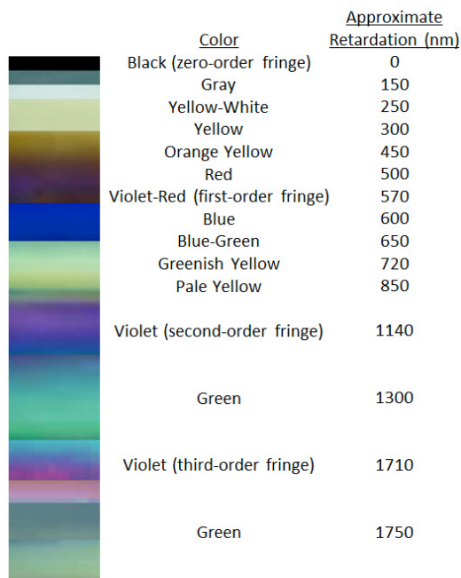
Figure 1: Fringe colors as a function of retardation, for the first 3 fringes. The color bar was generated by the authors, and color names and retardation levels were obtained from reference [1] and ASTM F218-13.
